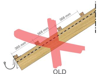
If roof pitch is between 15-30°, intermediate battens (not shown here) are obligatory to use. Please refer to Installation Manual, section Battens / Batten Spacing.
